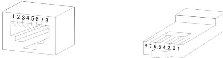
RJ-45 Connector pin signal:
