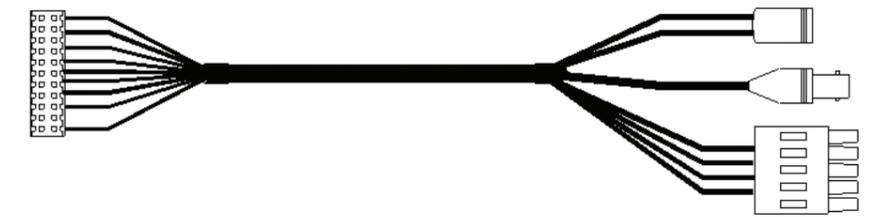
Data Cable for Power Supply, Video and Audio (DC 12V)
